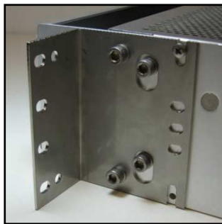
Fig. 1 – Mounting Bracket Position for ETSI Installation
