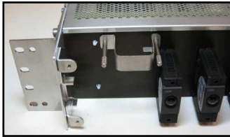
Fig. 12 – Removal Tool Location
