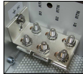
Fig. 9b – Common Return, grounded (B Side)
